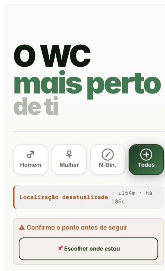
Figure 41 — Honesty in the client: “Localização desatualizada · ±154 m · há 106 s” and “Confirma o ponto antes de seguir” — staleness and positional uncertainty surfaced to the user instead of hidden: the offline/degraded discipline of Section 11.1 extended to the attendee's own position.
